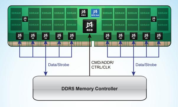
Notes: Here shows the application of SPD Hub on the DDR5 RDIMM as an example. This RDIMM contains Montage's DDR5 products (with an "M" logo) as listed below:
